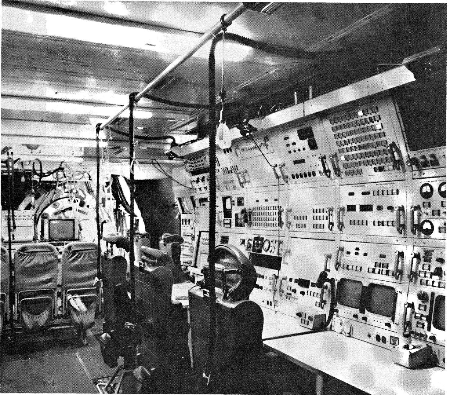
An inside view, looking forward, of the observing compartment. To the right is the telescope control console, where the flight engineer, mission director, and telescope operator work. Slightly visible forward of that is the tracker console. (The ADAMS is hidden in this view.) The three seats on the left are for the observers, facing their equipment rack. The round structure at the front is the telescope assembly, where the detector is mounted.
