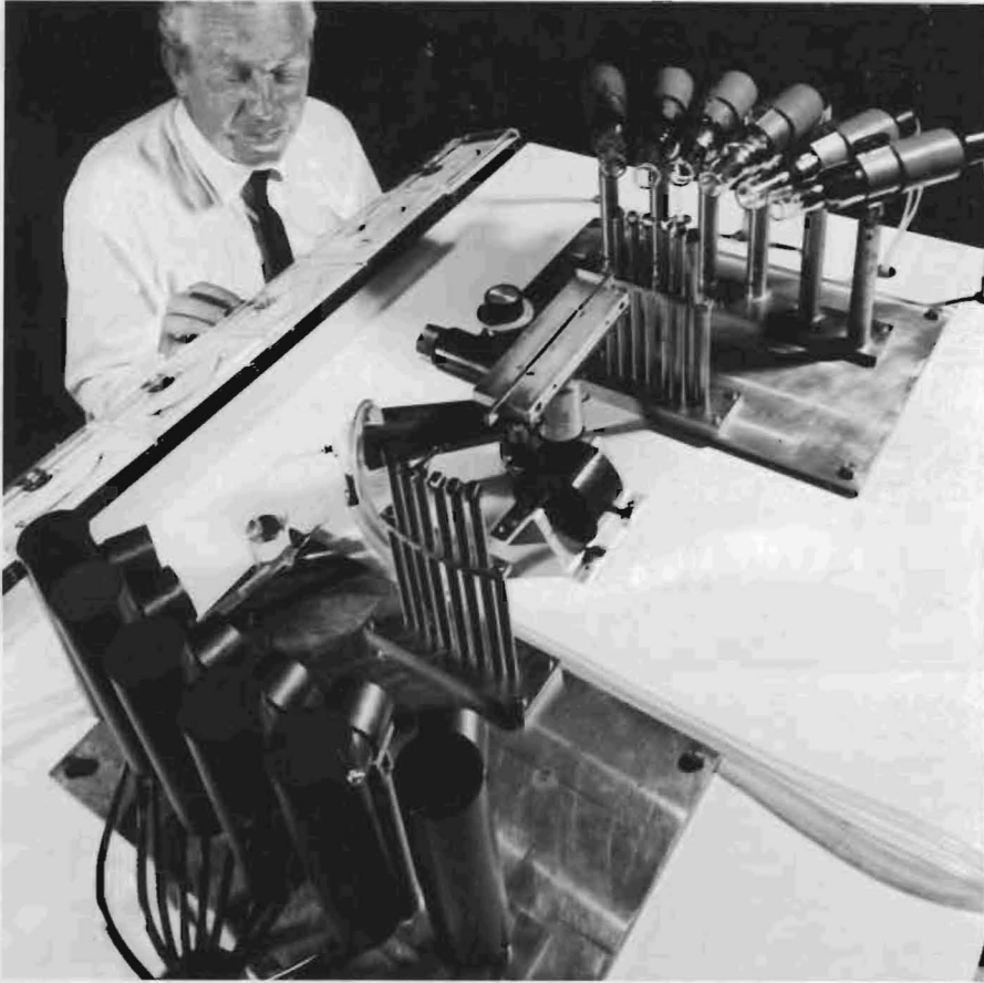
An experimental multichannel atomic absorption spectrophotometer for the simultaneous determination of six elements.
