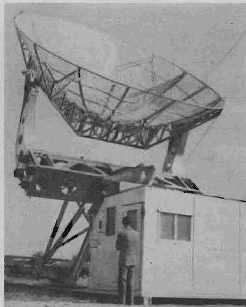
**This German Wurzbürger radar antenna has been adapted for use with Reber's equipment for receiving solar radiations and set up at Sterling, Va. Housing is German prefab steel shack.**
