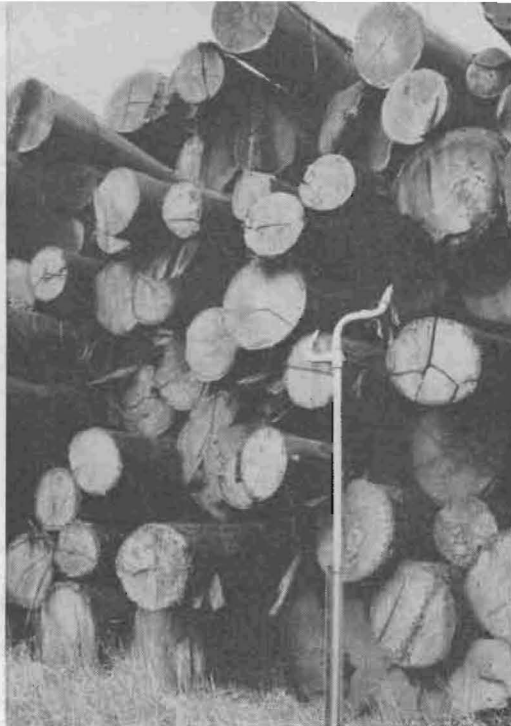
Fig. 2.—Only minor degrade is apparent in these logs, matched with those shown in Figure 1, after summer storage under water sprays.
