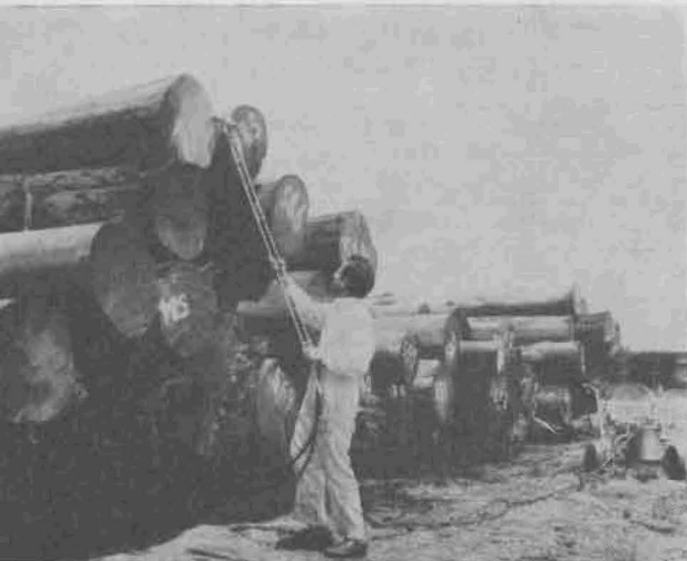
Fig. 4.—End coatings being applied by a lance attachment to a mobile pressure-pot spraying system.
