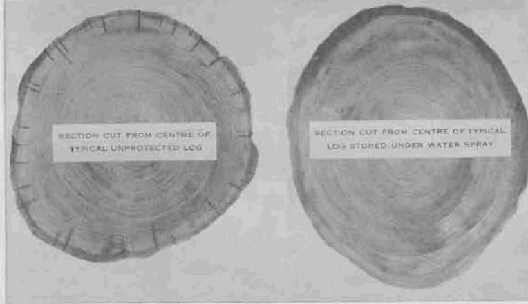
Fig. 3.—Cross sections of matched “ash” eucalypt logs showing: L.H.S., typical degrade developed during unprotected storage through a summer; R.H.S., high degree of protection provided by water sprays during storage through a summer.
