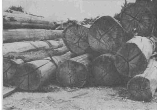
Fig. 1.—Typical degradation in unprotected “ash” eucalypt logs after summer storage.
