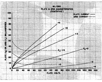
Figure 4 — ML-280 Tentative Grid Plate Characteristics.
