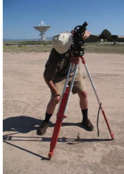
Fig. 33. Sullivan uses a 1940s era surveyor's transit to establish the locations of all markers and piers. The midday sun, used to determine true north, is at an uncomfortably high altitude. Photo: Goss.
