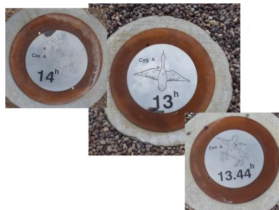
Fig. 22. Sample sidereal time markers for the radio sources Cassiopeia A, Cygnus A and Centaurus A. The sidereal time at which the disk would fall in the gnomon's "radio shadow" is indicated beneath a drawing of the traditional constellation (and its brightest stars) in which the source can be found. The exact location of the radio source within the visible constellation is indicated by a plus symbol. Each stainless steel disk is bordered by a beveled "rust-bloom" steel border. Photos: Sullivan.
