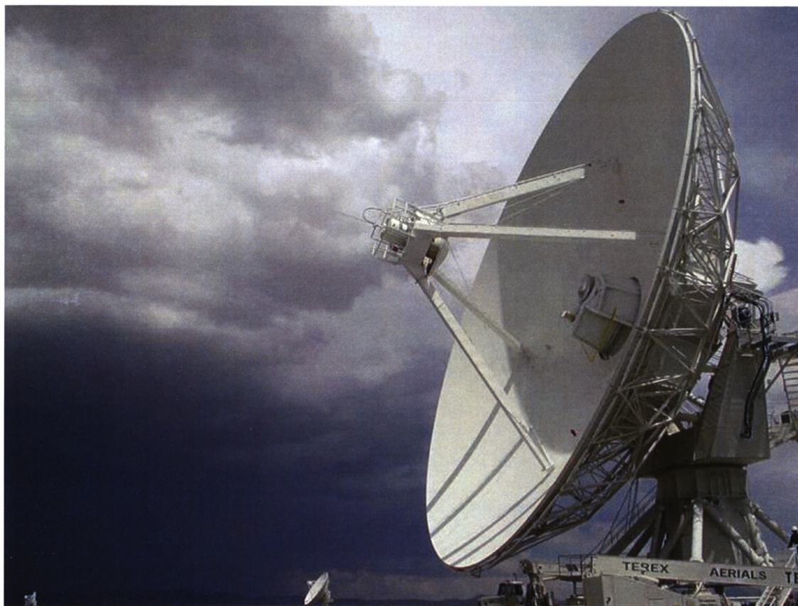
Figure A.1: The EVLA test antenna (VLA antenna #13) with its new feed cone installed in the middle of the reflector. This antenna is positioned on the VLA Master Pad for testing.
