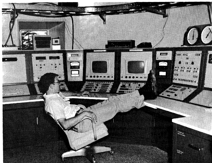
Fig. 5 - A local automotive mechanic demonstrates the new operator's position at the 140-ft, a position brazenly copied from the interferometer. The TV-like devices in the background are cathode-ray-tubes which display the coordinates of the telescope's beam and other information helpful to the operators.
