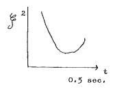
The resultant curve of \$\inspeces^2\$ as a function of time is shown. The first declining part of the curve is the classical damping; the second, rising part is the quantum excitation.
