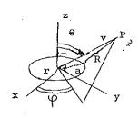
$$\overline{\Lambda} = \left(\frac{c}{c}\right) \int \frac{\overline{v}(\mathcal{T})}{R} \, d(\mathcal{T} - t + \frac{R}{c}) \, d\mathcal{T} \qquad \dots (1)$$
