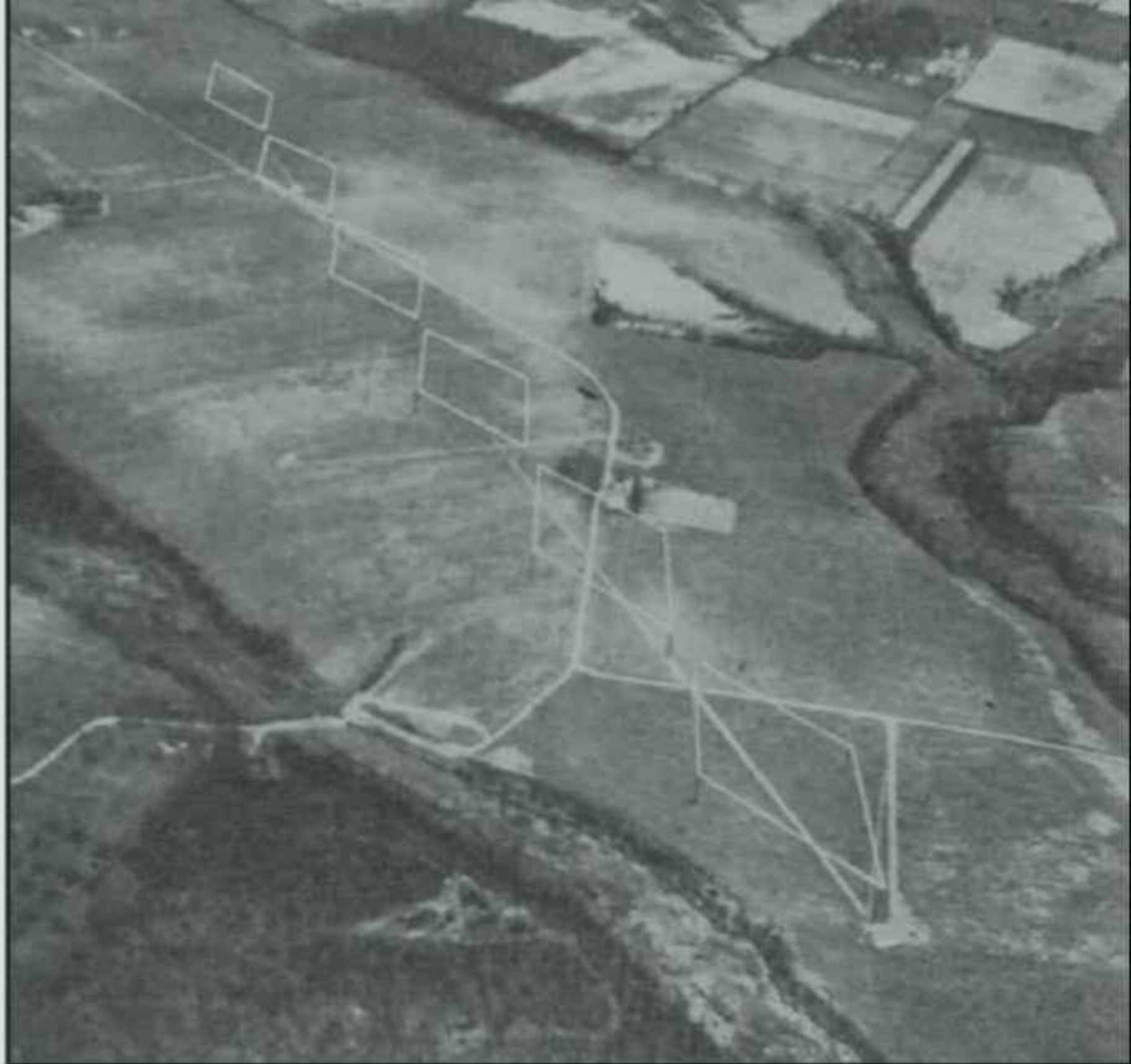
Fig. 2—Airplane view of the three-quarter-mile experimental MUSA on the receiving laboratory site located near Holmdel, New Jersey. The white line beneath the antennas is the newly filled trench in which coaxial transmission lines are buried. The building appearing in the right-hand foreground houses the receiving apparatus. The ground is flat to within \pm 4 feet.
