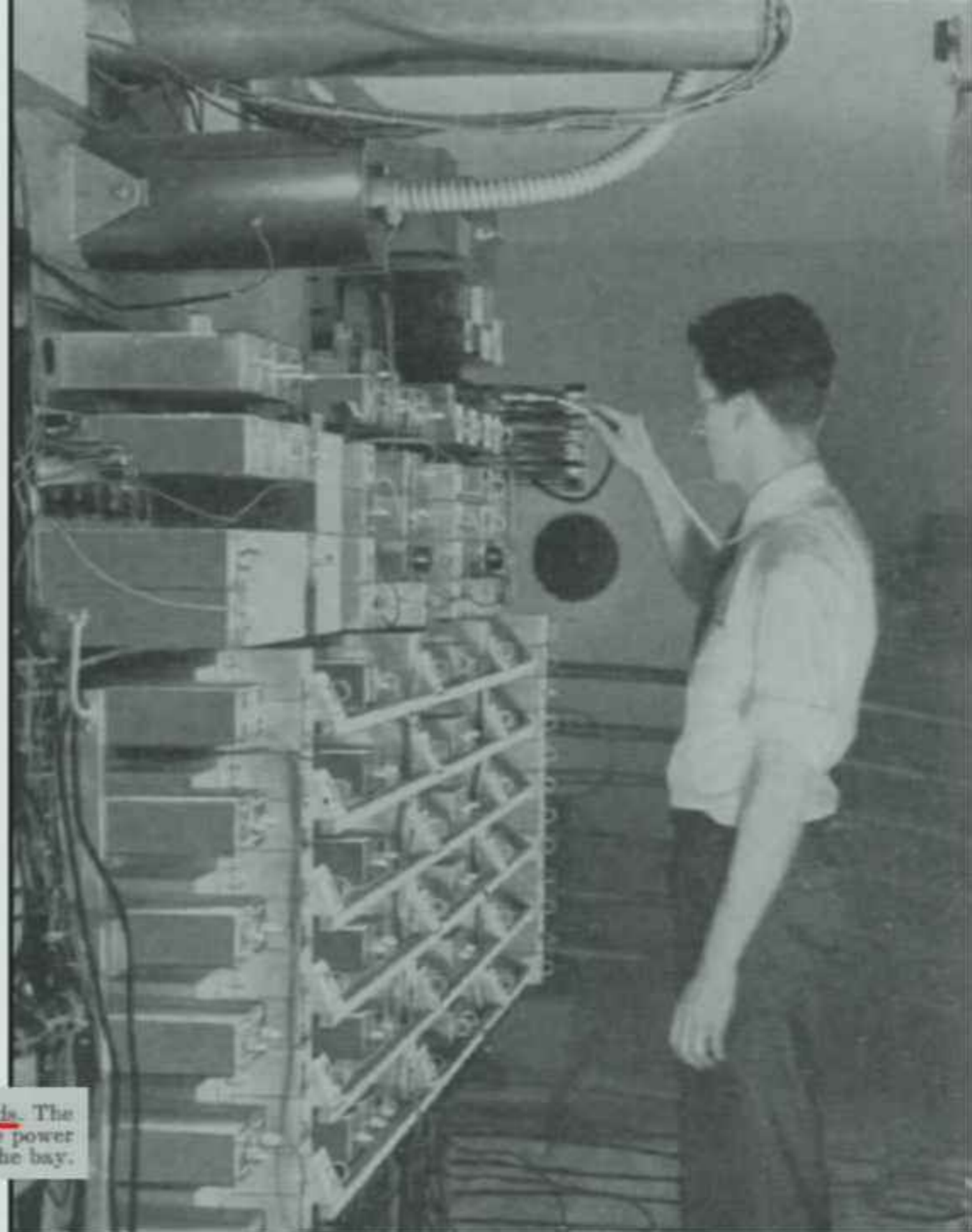
Fig. 18— Rear view of the receiving equipment. The six detector outputs feed the three branches via the square transmission lines.
