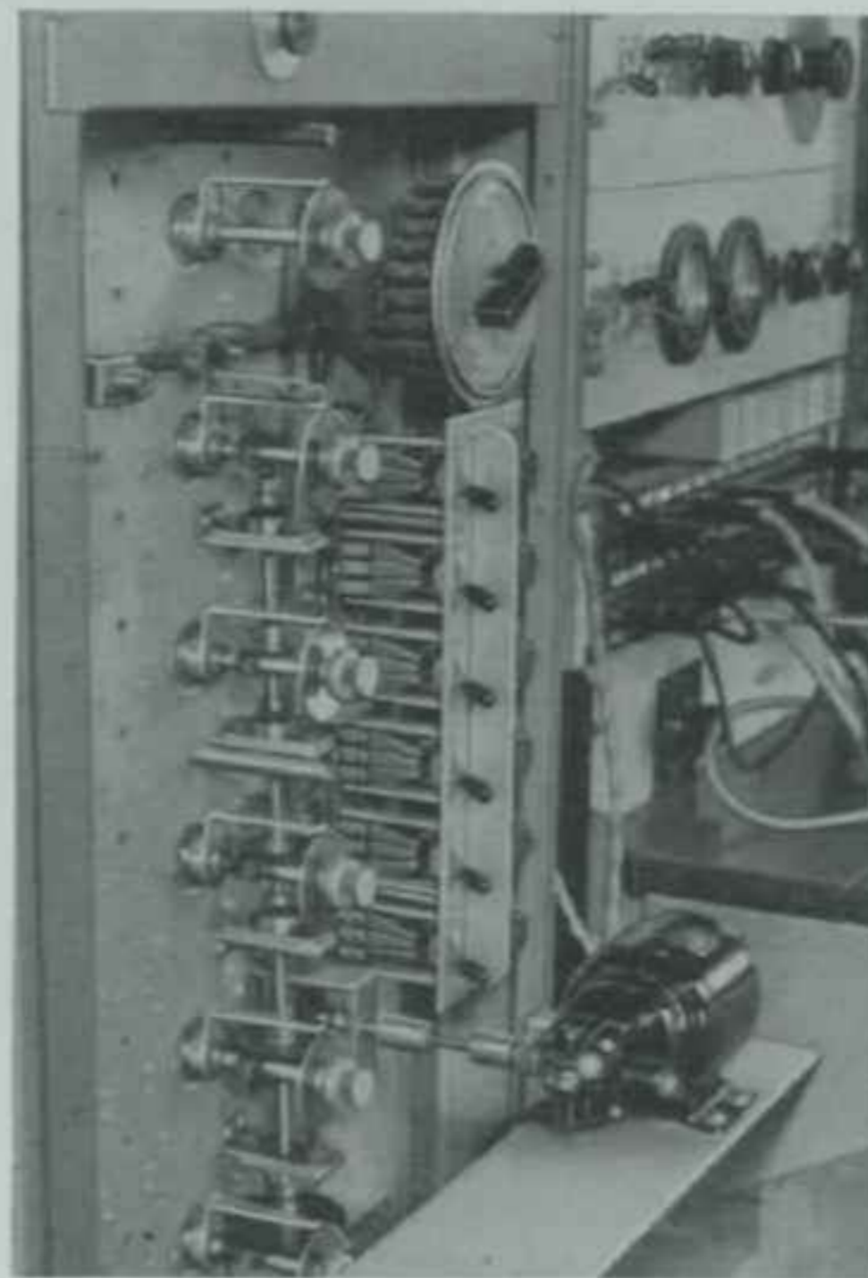
Fig. 15— Phase shifting panel of the monitoring branch. Only five of the six phase shifters are rotated for steering purposes. They are geared to the steering shaft in ratios of 1:1, 1:2, 1:3, 1:4, and 1:5.
