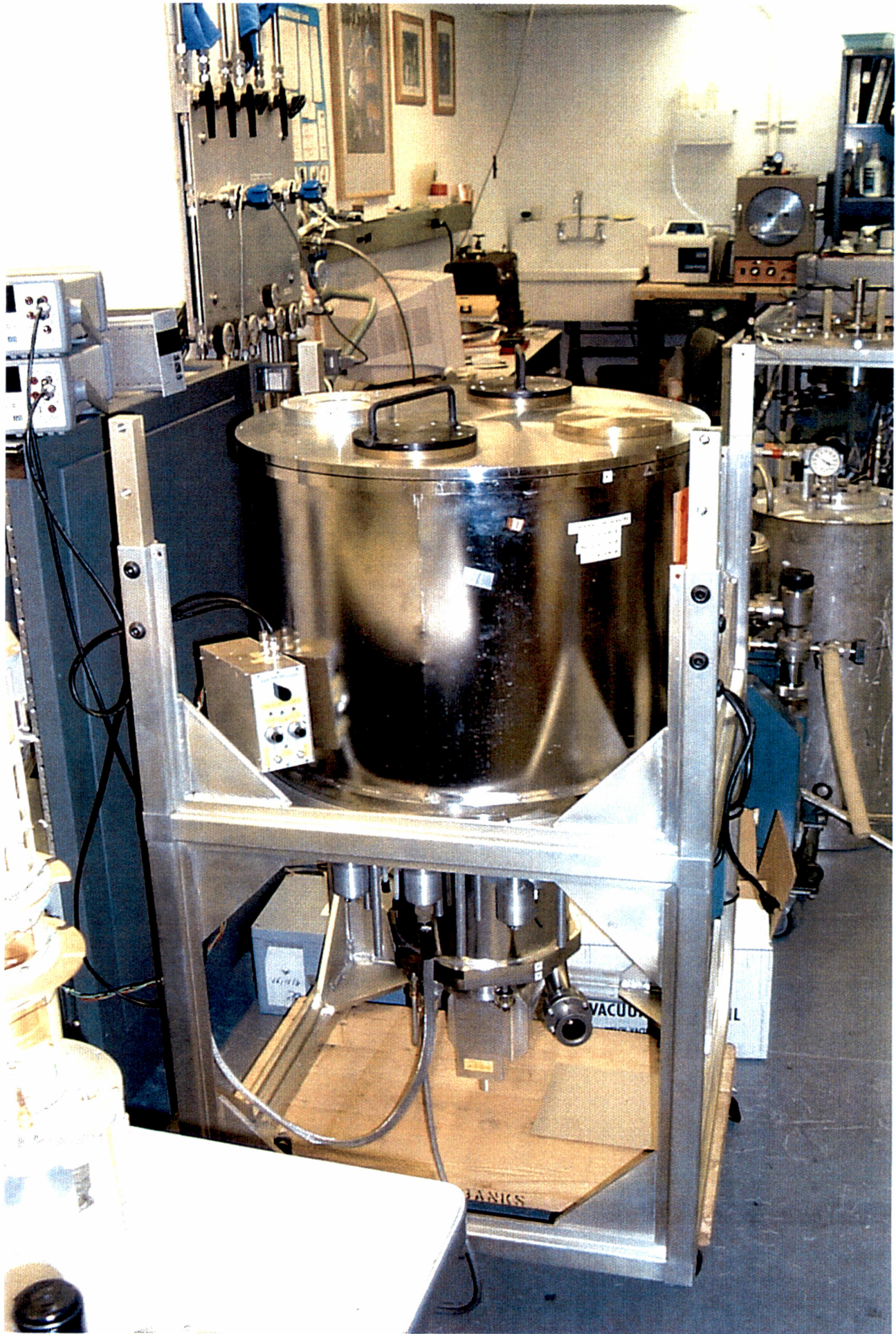
The receiver cryogenic dewar. The refrigerator can be seen mounted under the dewar.
