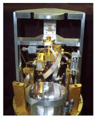
One of the 640 ALMA radio telescope receiver cartridges that operates simultaneously in two linear polarizations that are down-converted using a sideband-separating SIS mixer. Image credit: Neil Horner
