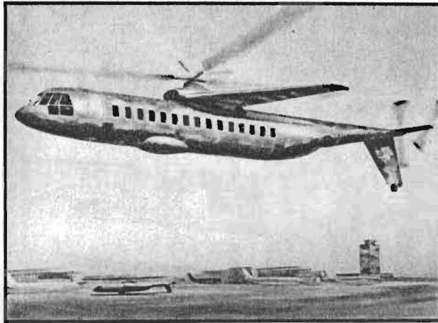
The Lockheed Company is currently looking at the possibilities of a 60-passenger air-bus, which they refer to as a "Metroplane." It could take off and land vertically, using its helicopter type rotor but travel the intermediate distance as a fixed-wing craft, with the rotor blades folded. Range would be in the 500-to-1,300-mile bracket.
