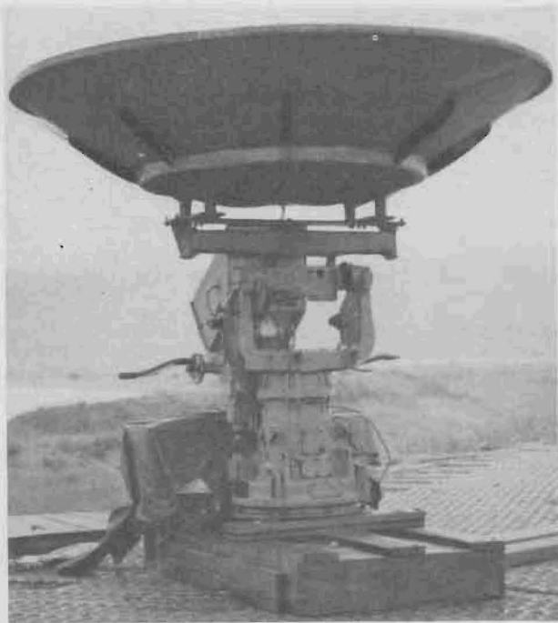
High-frequency radio waves from the sun were collected by this 10-foot radar mirror and focused on the antenna of a high-frequency receiver. Signals thus received were amplified and applied to an automatic recorder, providing charts of intensity versus time.
