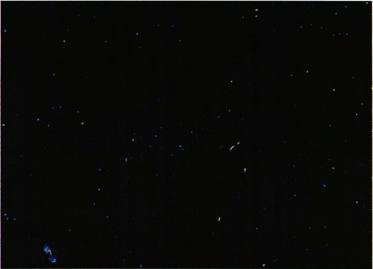
Figure 3.11: A 10.6 \times 7.7 arcmin 2 section of a deep ( \sim 120 hour) 1.4 GHz VLA image (rms noise \sim 3 \mu\text{Jy}/\text{beam} ); the resolution is \sim 1.5 arcsec, and the image shown is roughly a tenth of the full field-of-view. Such images will become routine with the increased sensitivity provided by the first phase of the EVLA Project. The New Mexico Array however will be able to actually image all these sources, providing \sim 10 beams across each source. This means that each of the pin-pricks in the current image will be resolved at roughly the level of the the extended, double-lobed source seen here in the southeast corner, aiding enormously in distinguishing AGN from starburst emission. Courtesy F. Owen (2003).
