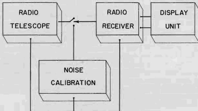
FIG. 1. The equipment used by radio astronomers.
