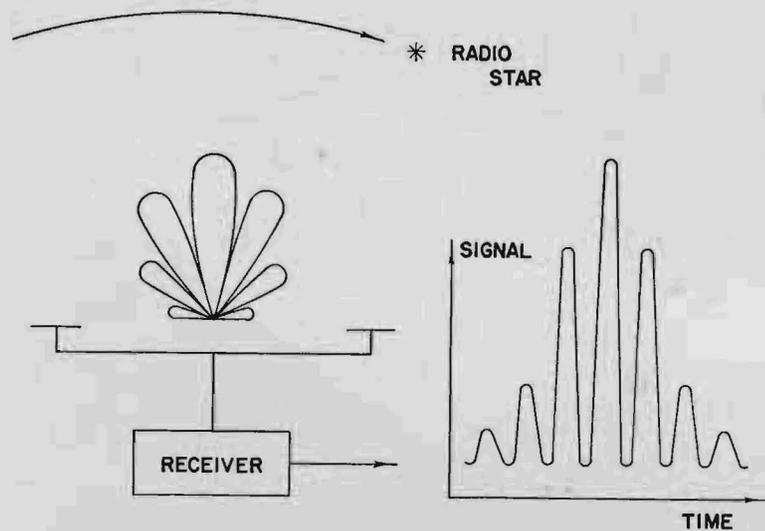
FIG. 3. A radio interferometer and the signal it produces when a radio star passes through the antenna pattern.
