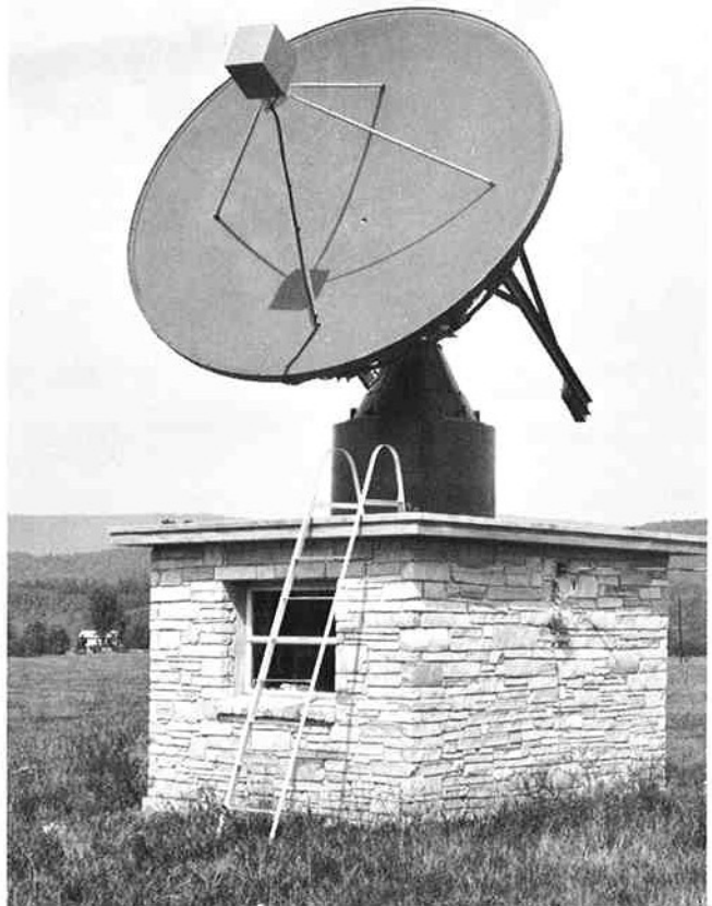
FIGURE 18. The 12-foot precision paraboloid that has the same f/d ratio as the reflectors of the 85-foot and 140-foot telescopes.
