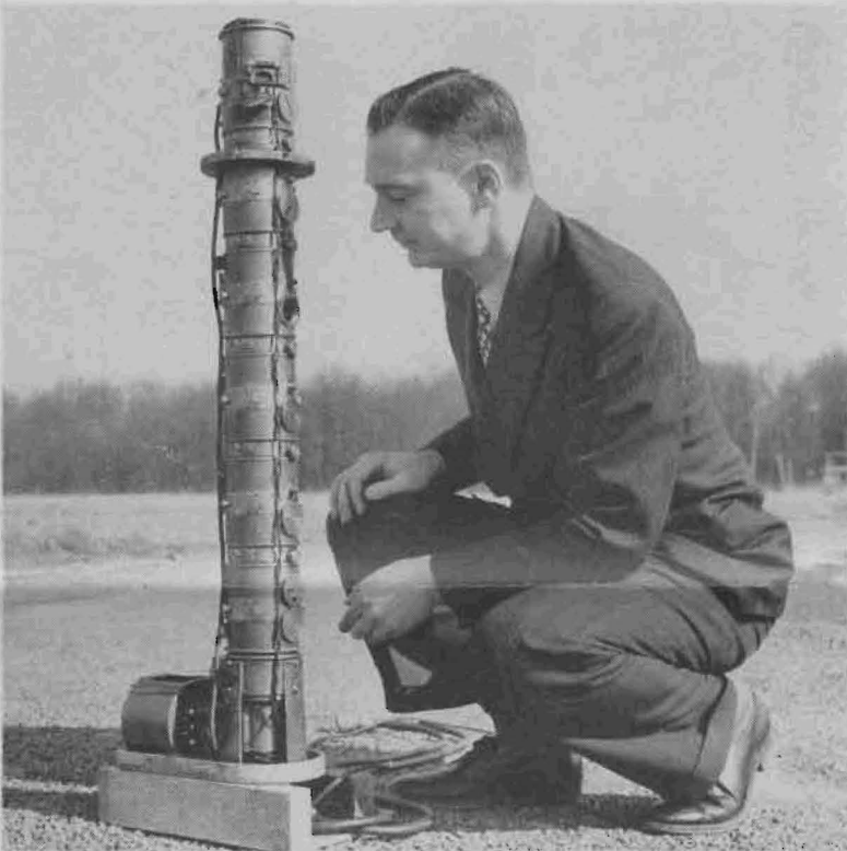
SPECIAL AMPLIFIER , which magnifies signals from stars 160 billion times into audible sounds or traces ( below ), is checked by Reber before installation.
