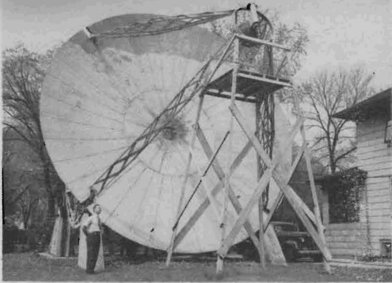
HOMEMADE RADIOMETER , built in 1937 by Reber in his Wheaton, Ill. backyard, picked up strong radio waves from the sun and parts of Milky Way.
