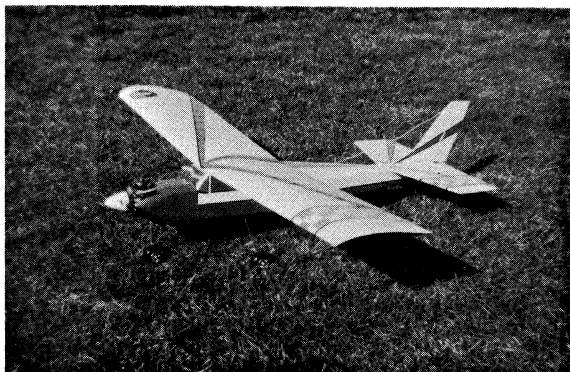
Jerry's three-channel, 50-inch wing-span Trainer. A good first airplane for multi-channel flying.
