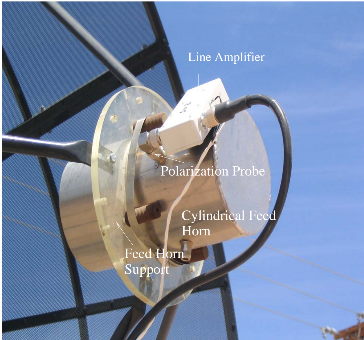
Fig. 8.— Feed horn, support, and line amplifier. The feed horn was designed based on the feed support of the 16ft dish. The horn can be moved back and forth through the middle of the support. This allows the telescope to be focused.
