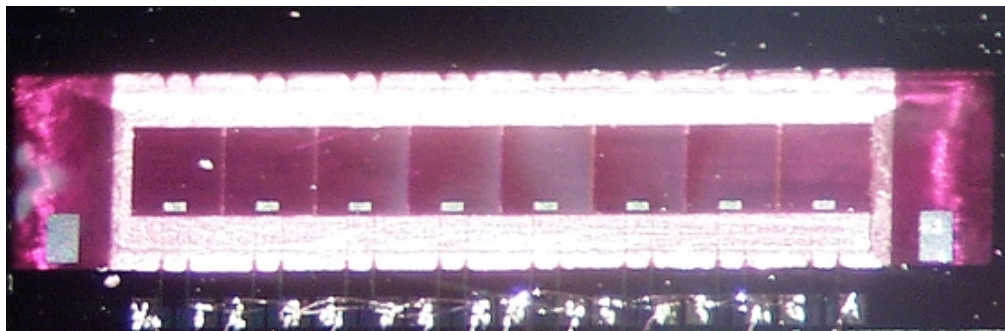
Figure 2. A single element from the middle of a linear array of TES bolometers. The absorber is 1mm on a side.
