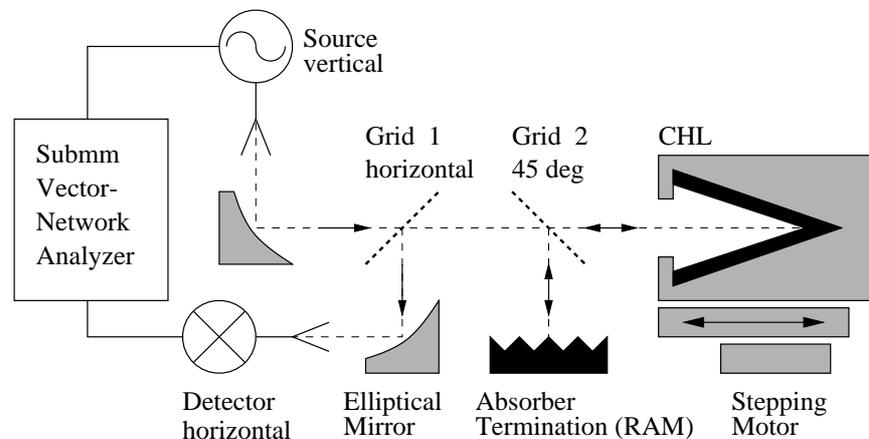
Figure 8: Setup of the quasi-optical reflectometer. Device Under Test is the CHL mounted on a motorized translation stage which allows to alter the phase of the reflected signal.
