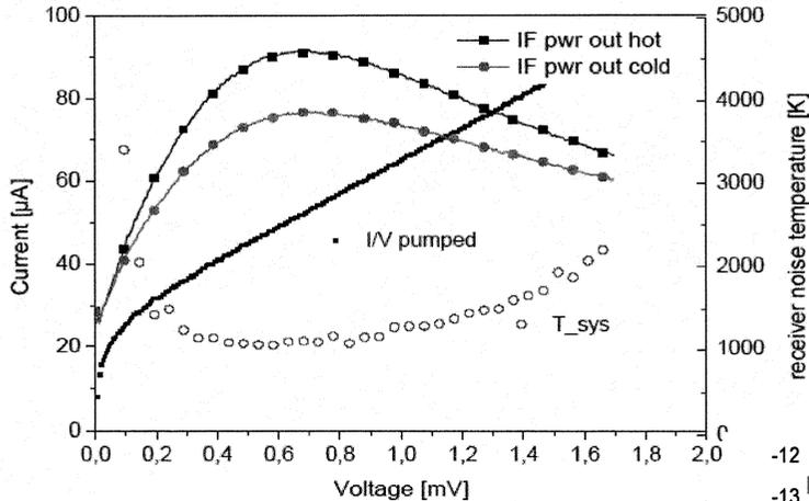
Fig. 6 Pumped IV curve (solid line). Hot and cold output (dots + line). Receiver temperature (dots).
