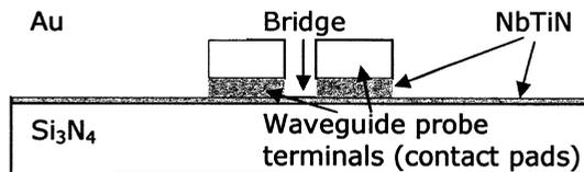
Fig. 1 simplified cross section of our HEB device
