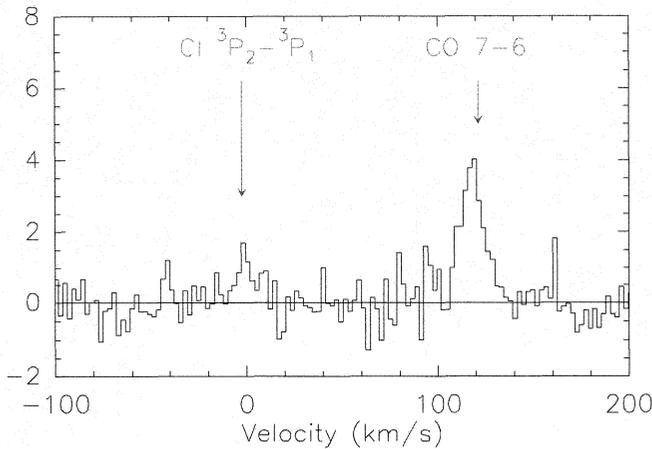
Fig. 8 Observation of DR21 with HEB mixer. The CO 7-6 line (right) lays in the lower band.
