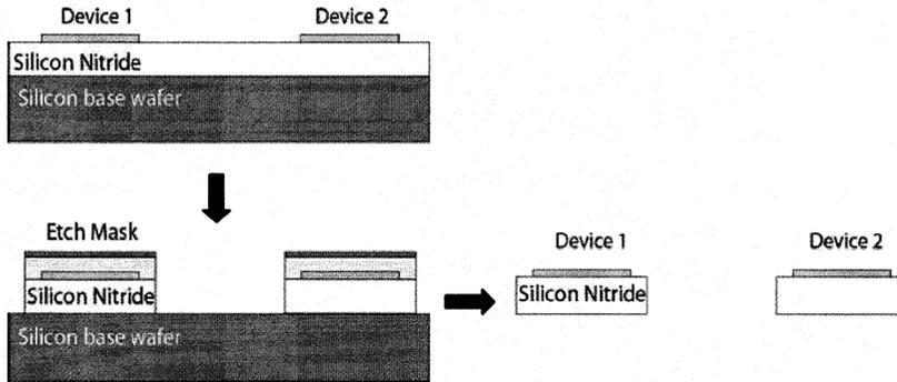
Fig. 2 Schematic description of the patterning and exposure of the Si<sub>3</sub>N<sub>4</sub> membranes
