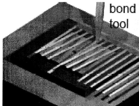
Fig. 3 Schematic description of bonding individual HEB device into the mixer block.
