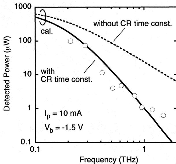
Fig. 7. Relationship between measured mm-/sub-mm-wave output power and frequency for the UTC-PD module.
