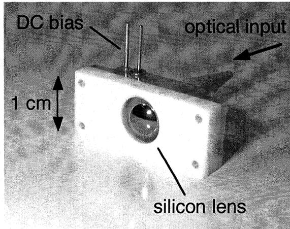
Fig. 5. Photograph of the fabricated quasi-optical UTC-PD module.
