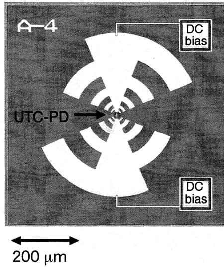
Fig. 1. Micrograph of the fabricated UTC-PD chip integrating a log-periodic toothed antenna.
