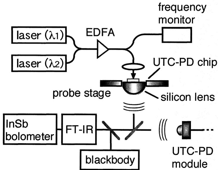
Fig. 2. Schematic drawing of the measurement setup.
