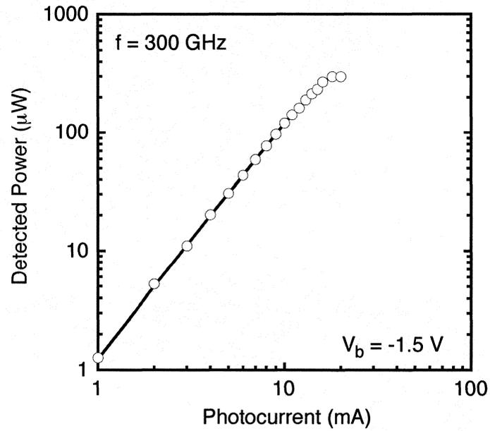
Fig. 3. Relationship between the measured mm-wave output power at 300 GHz and diode photocurrent for the antenna-integrated UTC-PD chip.
