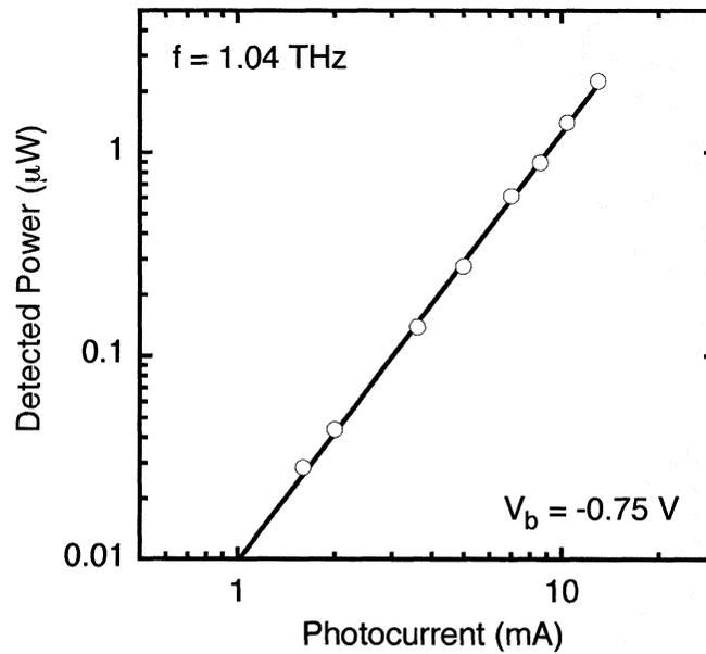
Fig. 6. Relationship between measured THz-wave output power and diode photocurrent for the quasi-optic UTC-PD module.
