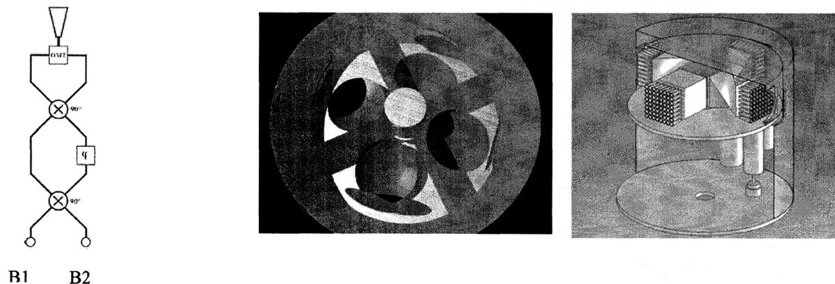
Figure 2: **Left:** Schematic view of the pseudo correlation receiver. **Middle:** A schematic view of a CLOVER telescope with four co-pointing Compact Range Antennas (CRA). Each CRA is fed by 64 horns. **Right:** The central cryostat containing four 64-feed arrays and the sections behind containing the hybrids and phase switches.
