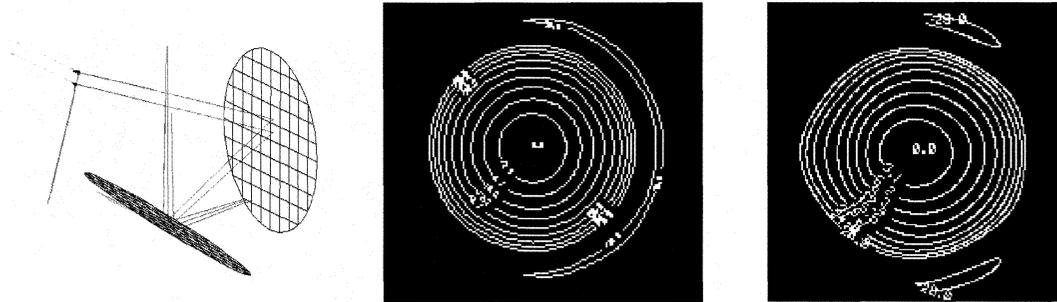
**Figure 3.** Radiation patterns obtained when the feed is placed in the centre of the array (centre) and with the feed is moved 50mm in the positive x-direction (right). The Physical Optics simulated geometry of the CRA (left) is also shown. The rays are shown for clarity but are not used in the calculations.
