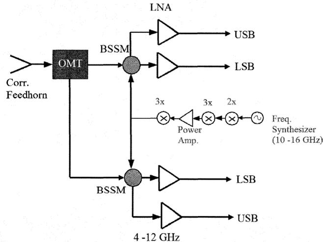
Figure 2: Schematic Block Diagram of 1mm SIS Receiver. See text for details of the receiver
