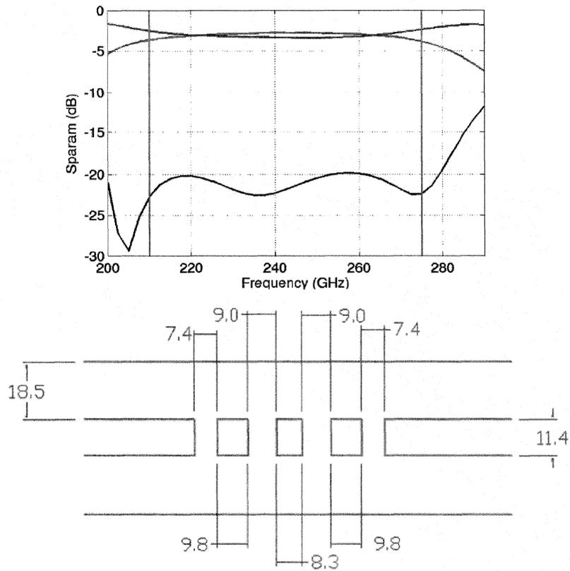
Figure 5: (a) Expected performance of the designed 4-branch line coupler. The designed band is 210 - 275 GHz. The red and blue curves show the coupling to the two output 3 dB ports, and the black curve shows the input match to the branchline coupler. (b) Details of the 4-branch line coupler. All dimensions are in mils. The width of the waveguides is 37 mils.
