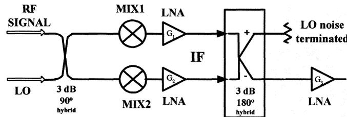
Fig. 1. Block diagram of the balanced mixer.
