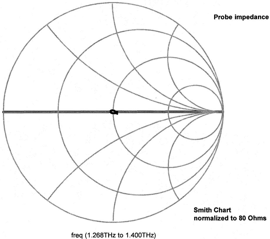
Fig. 8. The RF probe impedance at the HEB input is almost purely real of value about 80 Ohm between 1250 and 1390 GHz.
