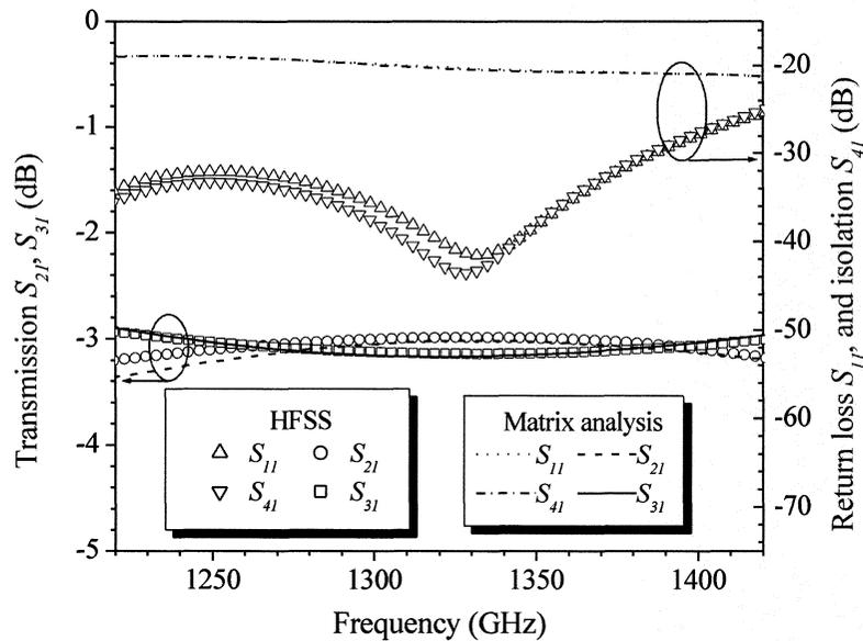
Fig. 3. Comparison of the results for magnitude of the hybrid S-parameters. Results of matrix analysis are shown by lines, results obtaining by HFSS<sup>TM</sup> simulations are demonstrated by open figures ( $\circ - S_{21}$ ,  $\square - S_{31}$ ,  $\Delta - S_{11}$ ,  $\nabla - S_{41}$ ).
