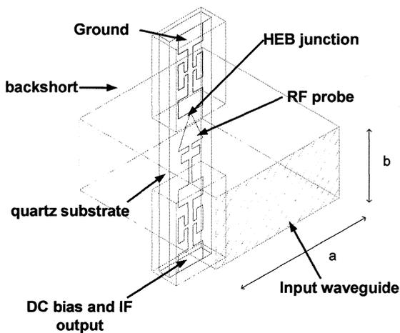
Fig. 7. Layout of the individual HEB mixer.
