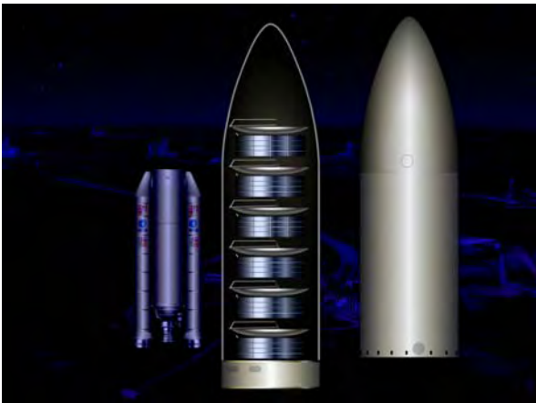
Fig. 1. The six elements of ESPRIT in an Ariane 5 faring. The telescope design has unfoldable subreflectors allowing dense packing and thus aiming for a single launch of the whole interferometer (artist conception).
