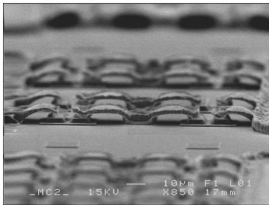
Fig. 8. SEM image of high power HBV diodes.
