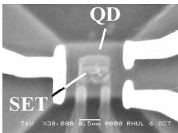
**Fig.1 SEM picture of the QD detector.**
