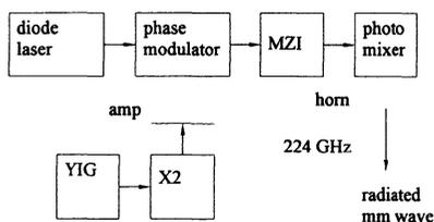
fig.1 open loop system
