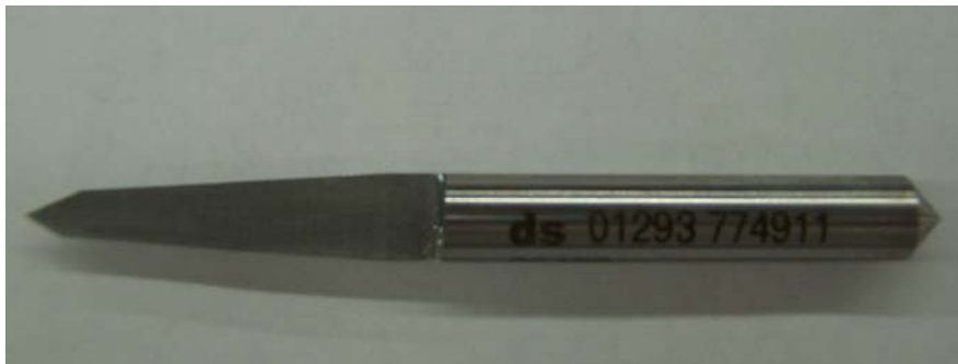
Figure 8: The tool used for machining the two-section, 230 GHz horn.
