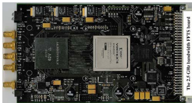
Fig. 9 Currently in development: The 2.5 GHz bandwidth FFTS. The board makes use of a first sample of E2V's 5 GS/s 8-bit ADC.
