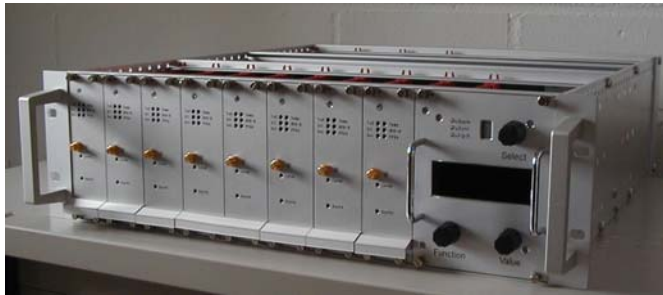
Fig. 5 Photograph of our 19 inch FFTS-crate, equipped with eight FFTS-boards and one FFTS-controller unit. The modular concept allows combining multiple crates to build large FFTS arrays.
