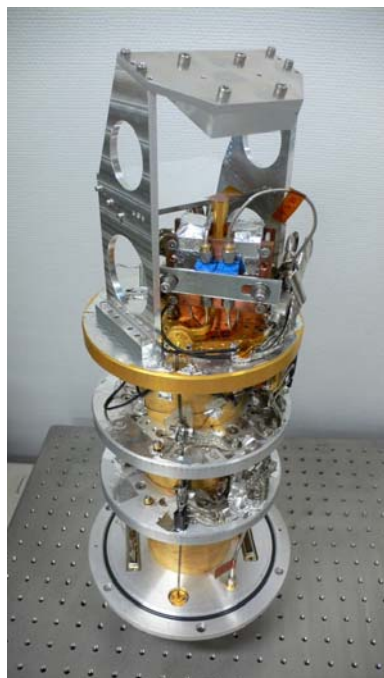
Fig.2 Whole image of CATS345. The height is about 400 mm. The diameter of the cartridge is 170 mm.
