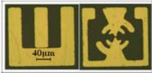
Figure 1. Microwave CPW (left) and terahertz LPA1 (right) structures for coupling to the CNTs.
