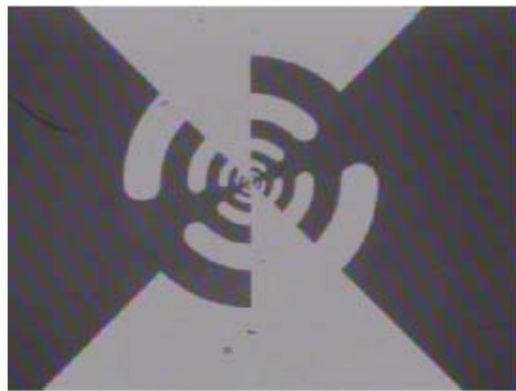
Figure 2. LPA2 with 1 μm gap used in later THz measurements.
