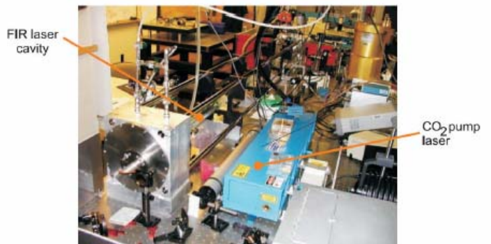
Figure 11. The \text{CO}_2 -laser pumped THz gas laser
