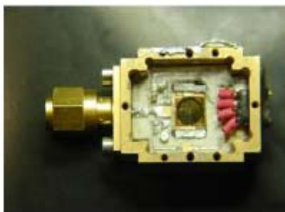
Figure 8. The fixture used for THz measurements. The device chip is in the center of the fixture and the silicon lens on the opposite side (visible through the sapphire substrate).
