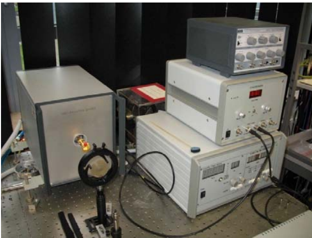
Fig.20 Experimental setup. 300 GHz BWO with an output power \approx 20 mW (multimode) and the SL-Tripler providing output power \leq 1 \mu W at frequencies up to 1 THz.
