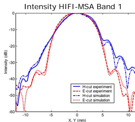
Fig. 3 Simulated and measured intensity along the E- and H-planes of the maps in Fig. 1 and 2.
