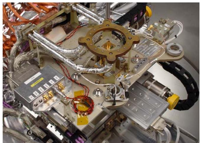
Fig. 7 View on the vacuum scanner system. In the centre the horn of a coherent test source and the thermal interface to the cold absorber screen are visible.
