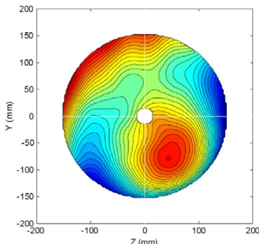
Fig. 14 Example of a measured wavefront error map in band 1.
