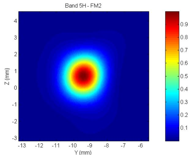
Fig. 10 Reconstructed focal plane field distribution in band 5H.
