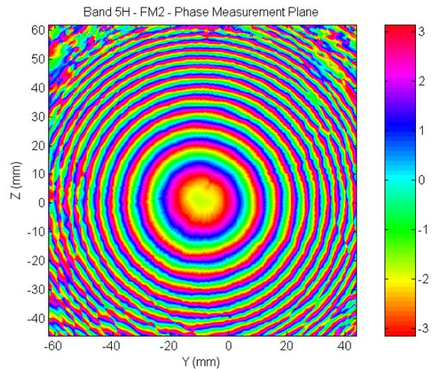
Fig. 9 Measured phase distribution of band 5H.
