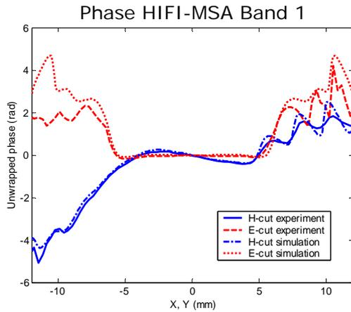
Fig. 4 Simulated and measure phase cuts of MSA band 1 at 480 GHz.
