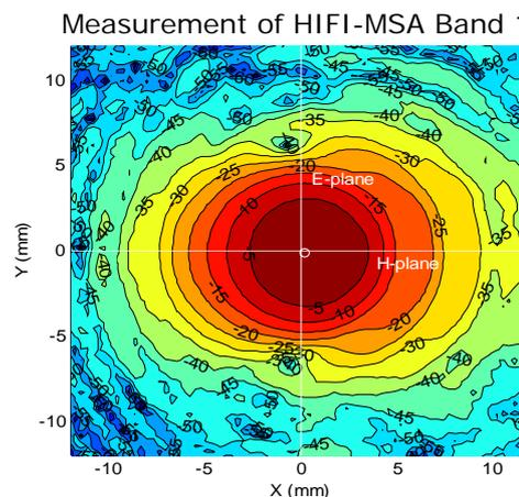
Fig. 2 Measured beam pattern of HIFI MSA band 1 at 480 GHz.
