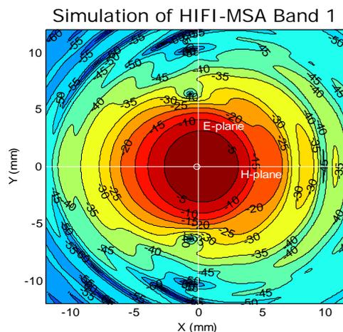
Fig. 1 Simulated beam pattern of HIFI MSA band 1 at 480 GHz.
