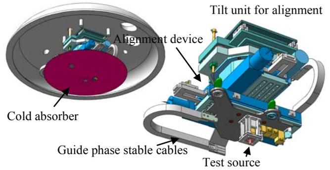
Fig. 5 Artist impression of vacuum scanner system used for the measurement of the focal plane beams of HIFI.
