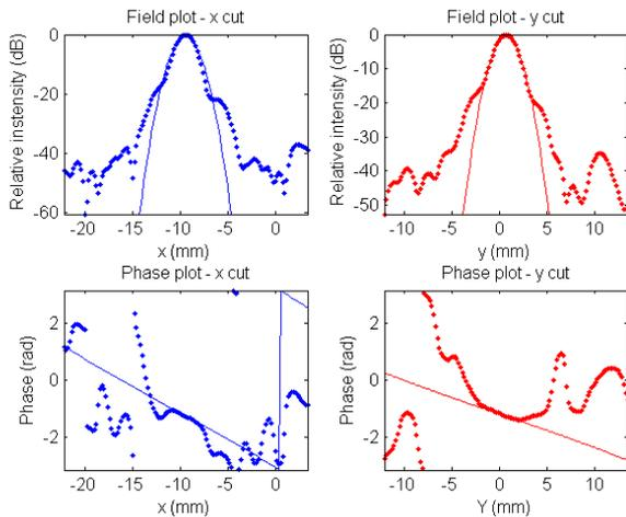
Fig. 11 Measured and fitted intensity and phase cuts in the focal plane for mixer band 5H.
