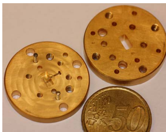
Fig. 4 Two-piece waveguide block halves for the 202 GHz quintupler. The AlN microstrip circuit is mounted in the waveguide channel of the block half on the left. A 50€ cent is included for size comparison.
