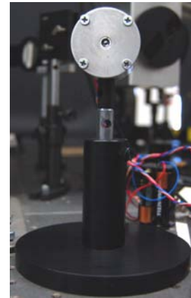
Fig. 4 Picture of the THz detector composed of the silicon lens, InGaAs asymmetrically shaped diode, and low-noise preamplifier. The detector is suited for free space experiment. The preamplifier is sourced from four AA-size alkaline batteries.
