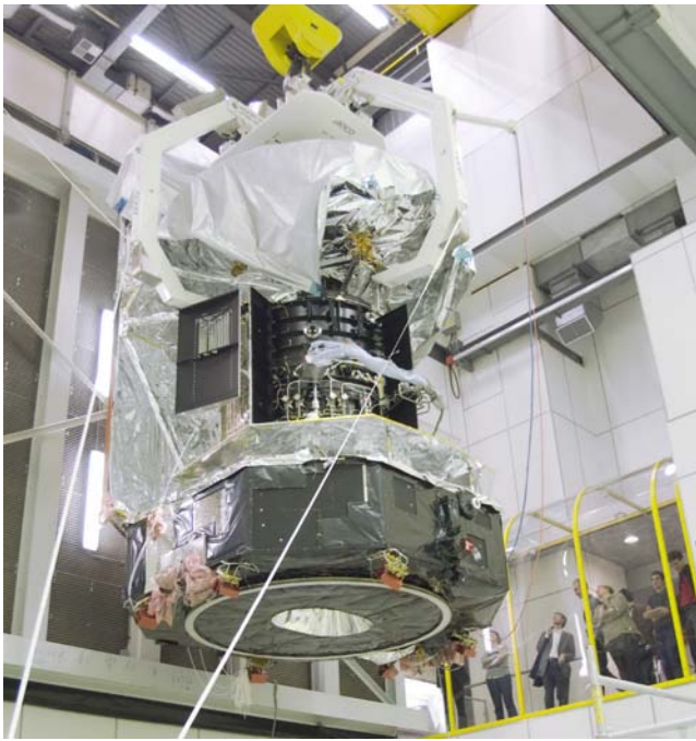
Fig. 1. Herschel lifted to be placed into the LSS. The 3.5 meter telescope is covered by a protection cloth. The rear side of the solar panel is covered by multilayer thermal insulation (MLI) blankets. The black central cylinder contains the 2500 liters He and the focal plane units of the instruments. The lower section, covered with black MLI contains the warm electronics that will be kept at room temperature by their own dissipation. Clearly visible is the LO radiator close to the solar panel, this will allow the LO to cool to 125 K in flight.
