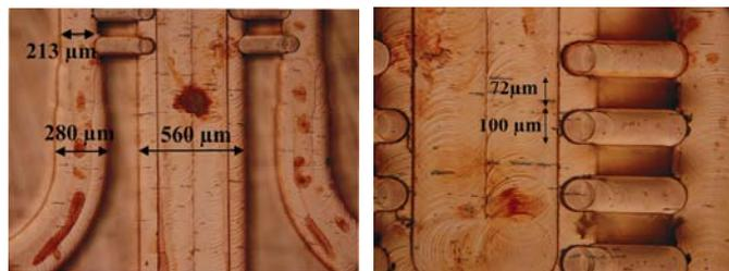
Fig. 10. Detail of the three metal “teeth” between branchline slots of one of the coupler sidearms.
