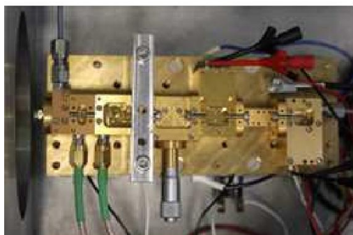
Fig.1. Top: vacuum RF test chamber developed to test receiver in the -20 to +45^{\circ}\text{C} range (left), and 664 GHz receiver under test (right). Bottom: DSB mixer conversion losses measurements of 664 GHz (left) and noise temperature (right) over this temperature range.
