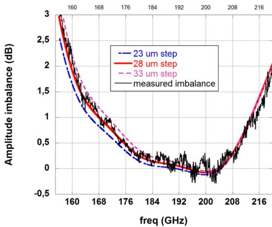
Fig. 4. Simulated performance for different step length lengths.
