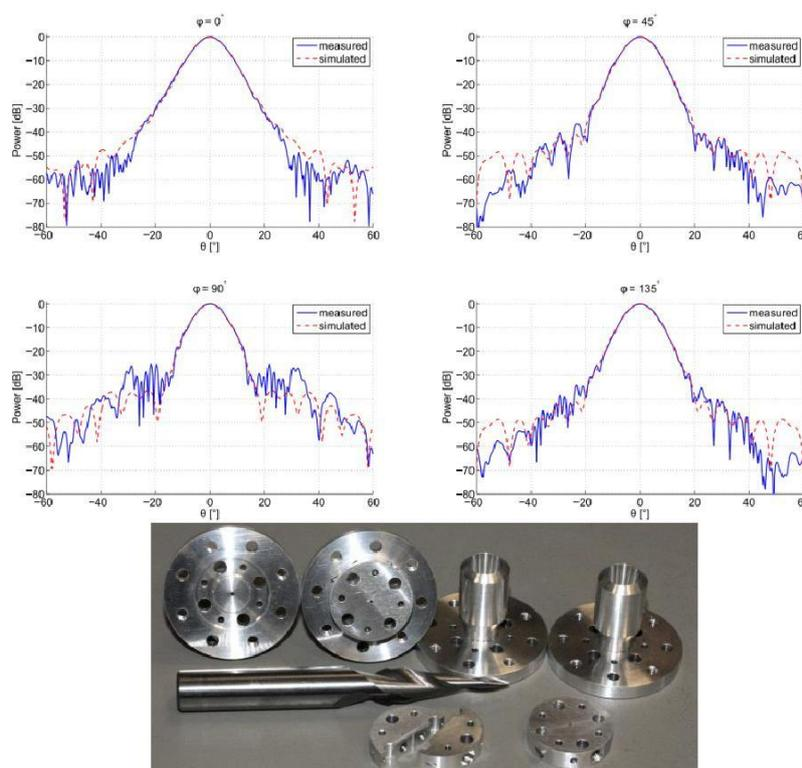
Figures showing beam patterns in four different cuts from measurements (solid lines) and simulations (dashed lines) and a photo of four prototype feeds, rectangular to quadratic waveguide transitions and the custom-made broach used for manufacturing the feeds.
