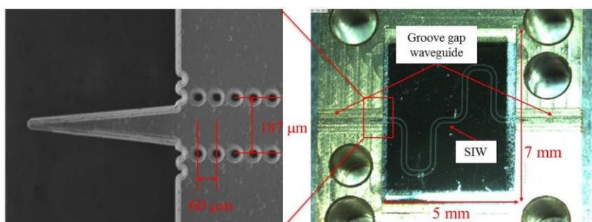
Fig. 1 A scanning electron microscope image of the SIW and optical microscope image of the test fixture including the SIW.
