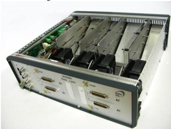
Fig. 6 NOEMA laser emitter rack.
