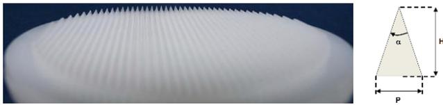
Fig. 1 *Left*: HDPE vacuum window showing the triangular grooves on one of the surfaces. *Right*: Geometry of the corrugations.
