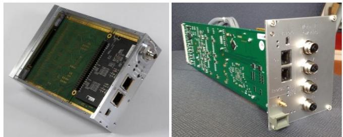
Fig. 7 Ethercat modules for *left*: biasing the NOEMA SIS junctions and *right*: controlling the warm IF chain and laser rack emitter.
