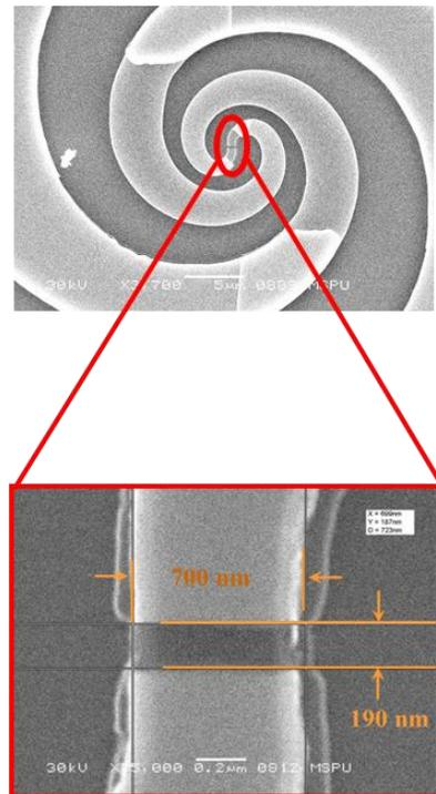
Fig. 4 SEM image of the antenna type A.
