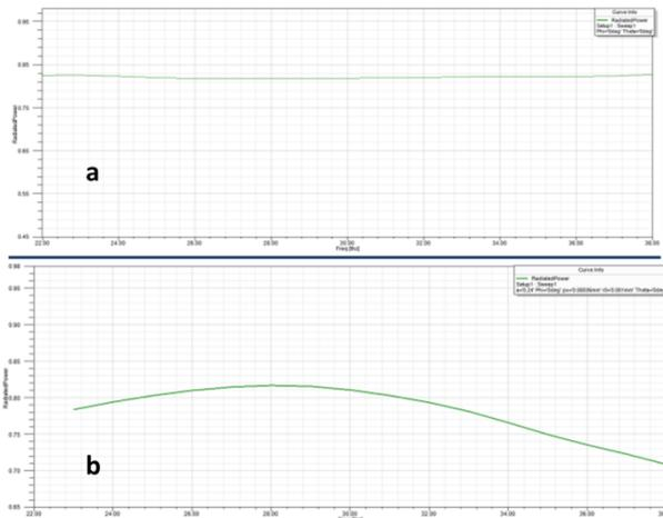
Fig. 3 Simulated efficiency the antennas vs. frequency.
