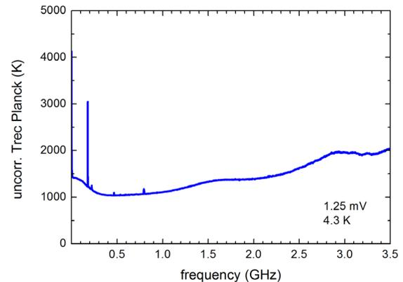
Fig. 1 Uncorrected DSB Trec(IF) (Planck) for a HFA flight mixer candidate at a LO frequency of 4785 GHz. A 5  $\mu\text{m}$  thick Mylar beamsplitter in vertical polarization was used as diplexer with a fully evacuated signal path. No corrections for signal path losses were applied (beamsplitter  $T=70\%$ , dewar window  $T=92\%$ ) were applied. The spurs at low IF originate from the QCL local oscillator.
