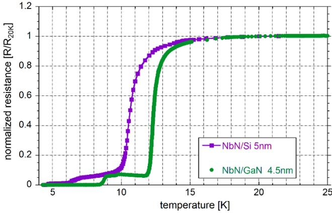
Fig. 1 Resistance versus temperature curve of the HEB bridges made of NbN, which was grown onto Si substrate ( $T_c=10.5$  K) and GaN buffer-layer ( $T_c=12.5$  K). The double transition is caused by the weakened superconductivity under the contact pads.
