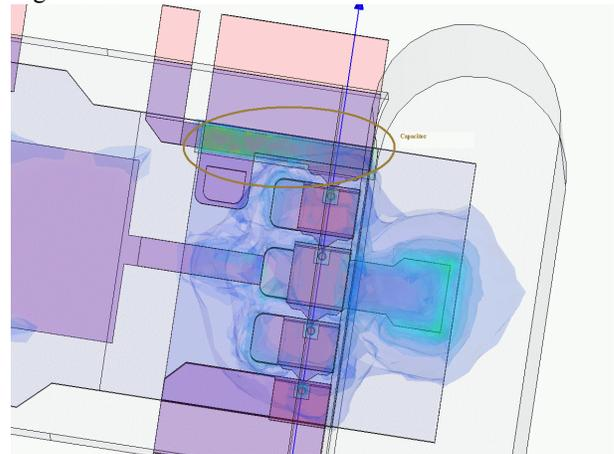
Fig. 1 The tripler shown with gold straps to the CVD diamond. The area circled is a single-layer capacitor for DC bias. Contours are 600GHz E-field
