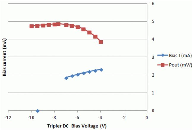
Fig. 8 Measured output power (at 610GHz) vs. DC bias, showing output power (red) and rectified DC bias current (blue)
