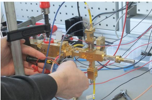
Fig. 6 Double-directional coupler and harmonic mixers, providing full input match characterization (similar to a VNA)
