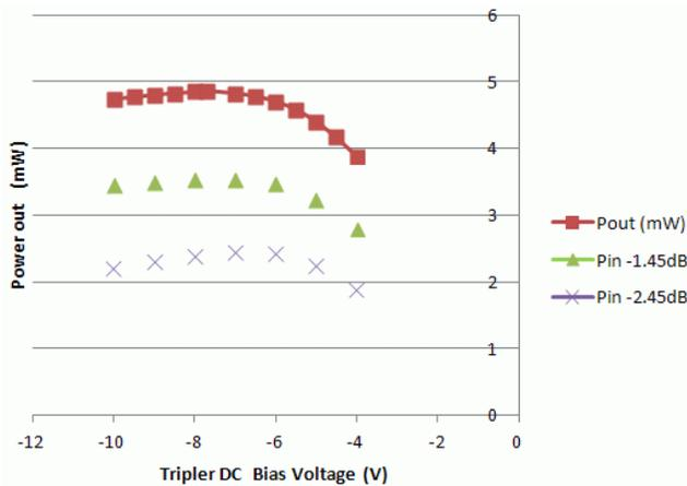
Fig. 9 Power output vs. Bias voltage plotted for different input powers
