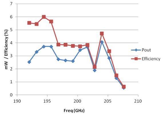
Fig. 7 Plot of measured Output power (blue, mW) and Efficiency (red, %). Frequency scale is for the tripler input.
