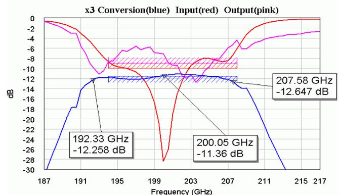
Fig. 2 Simulated conversion efficiency and input and output match (dB scale) for an input power of 100mW and 10V bias
