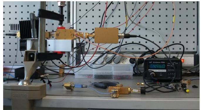
Fig. 7 For output power measurements, the PM4 meter is directly connected to the tripler using a taper-transition to overmoded WR10.
